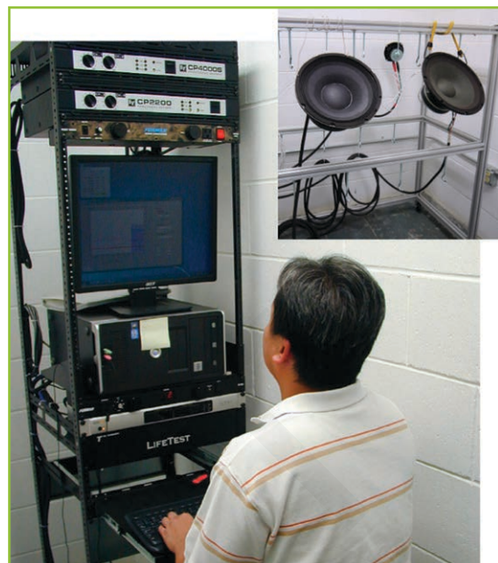
MISCO's Power Test Chamber with custom software assures reliability. The inset photo shows speakers during the testing process.
