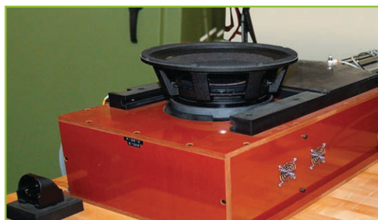
The massive 3.4-kilojoule Magnetizer is used for large neodymium or ferrite magnet structures.
